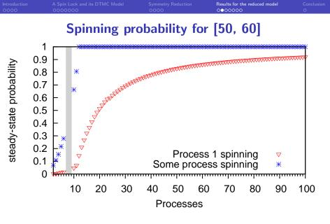
model generation fails for 7-9 processes because of a 190 GB RAM limit
